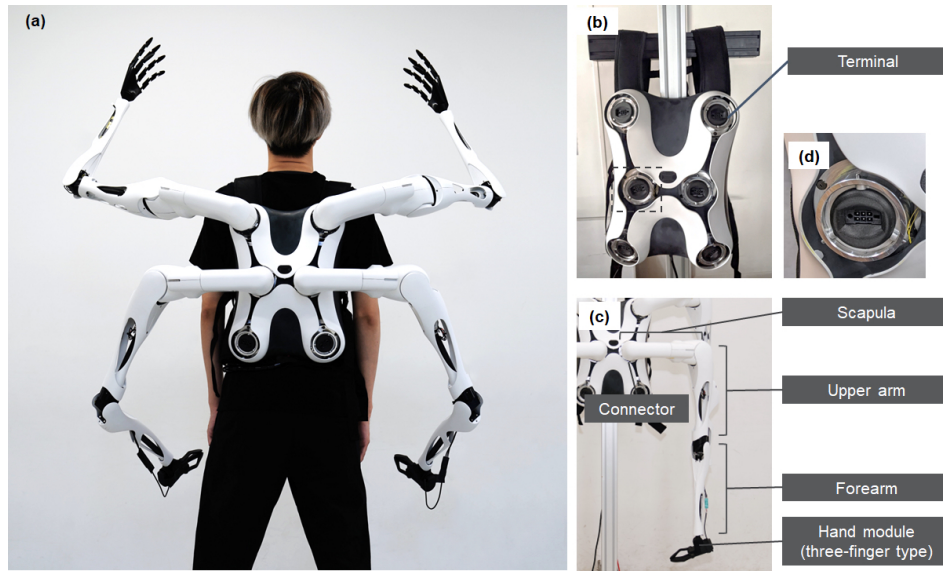
Figure 16: Appearance of the JIZAI ARMS. (a) The JIZAI ARMS being worn. (b) The base unit with six terminals for mounting the robotic arms. (c) A robotic arm with a three-fingered hand. (d) A terminal on the base unit. Magnified view inside of the dotted line of (b).
