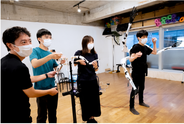
Figure 10: Three operators shared the controller and manipulated three arms respectively.
