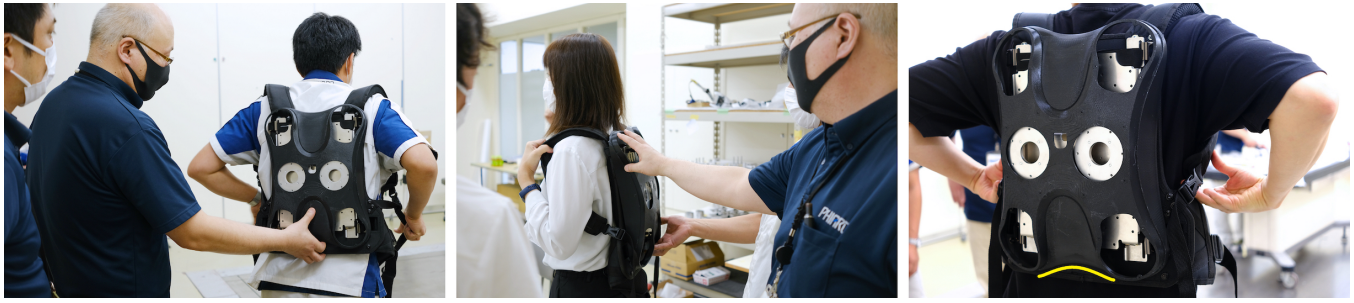
Figure 8: Each member with a different physique tried on a current prototype of the base unit and identified necessary modifications. We also decided to remove the part (yellow lined in the right picture) to improve the appearance.
