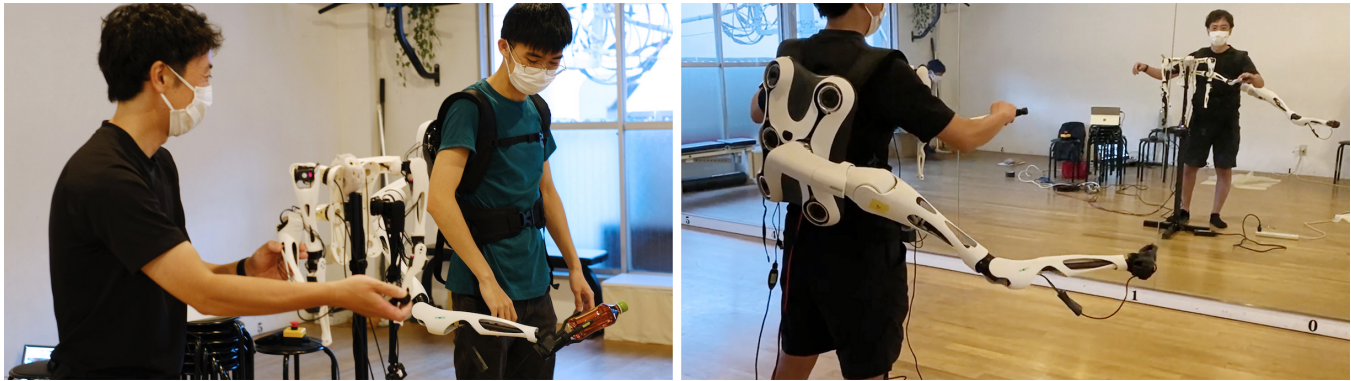
Figure 9: Left: An operator operates a wearer’s robotic arms. Right: A wearer operates the worn arm himself.
