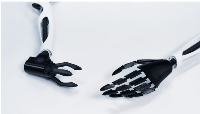
Figure 18: Hand modules. Left is the three-fingered manipulator. Right is the five-fingered hand.
