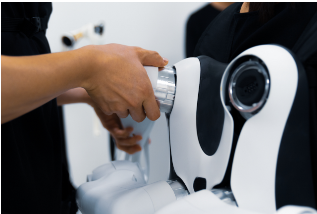
Figure 11: A person is detaching a robotic arm from a terminal of a wearer's base unit.
