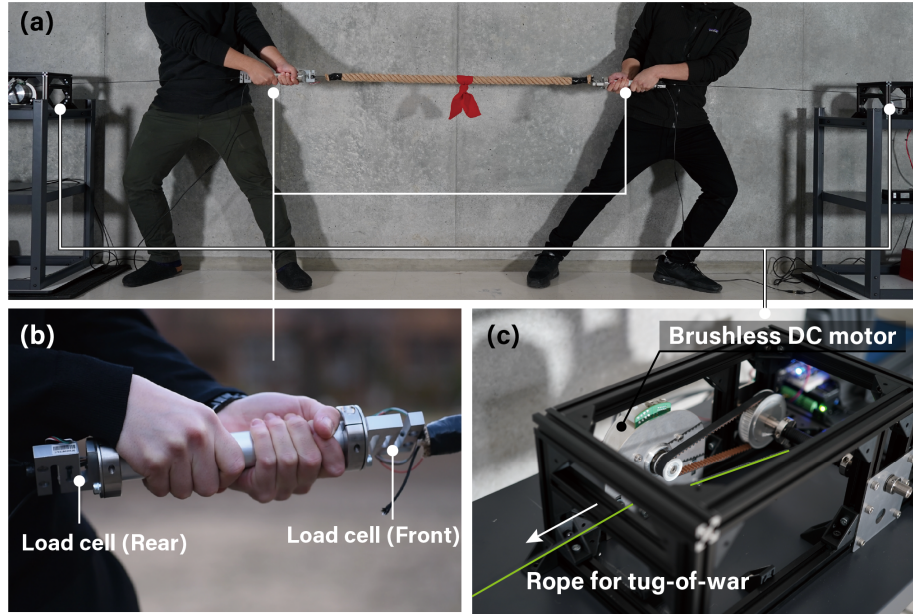
Figure 2: (a) BPs pull at the rope using the handle device. (b) The handle device has two load cells to measure forces at both the front and rear ends, which detects how each player is applying force. (c) A brushless DC motor can pull at the rope from behind each player.
