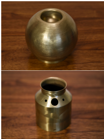
Figure 3. Brass made enclosure (top: outside, bottom: inside)
